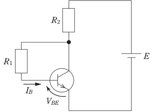
1.  $I_B \doteq \frac{E - V_{BE}}{R_1 + h_{FE}R_2}$
