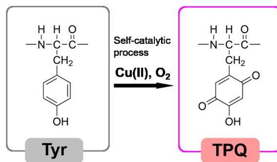
Fig. 1 Self-catalytic TPQ biogenesis
